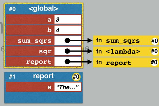
Since a is unknown within the local frame, Python checks the parent frame.
